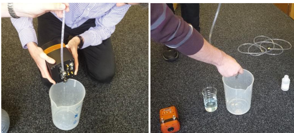
Figure 2: Drain the camera after use (left) and drain tubes (right)
